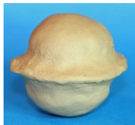
Figure 9. Clay simulation of a cast ball-shaped flan with seam.
