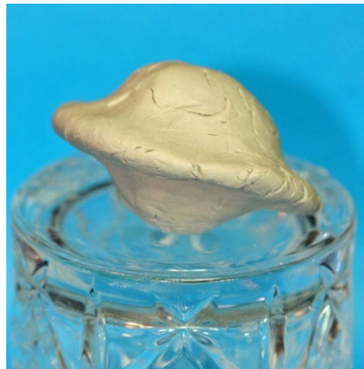
Figure 21. Cast flan ball placed on bottom die with the casting seam not perpendicular to the die face.
