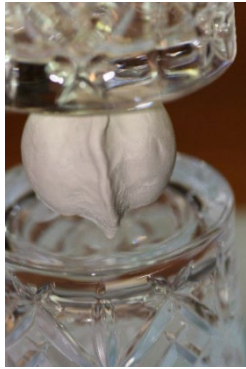
Figure 10. Placement of the flan ball between the obverse and reverse ‘dies,’ with casting seam perpendicular to the die faces.
