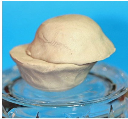
Figure 25. Flan with casting misalignment placed between dies with seam parallel to the die faces.
