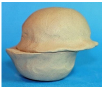
Figure 24. Flan resulting from mis-aligned halves of the casting mold.
