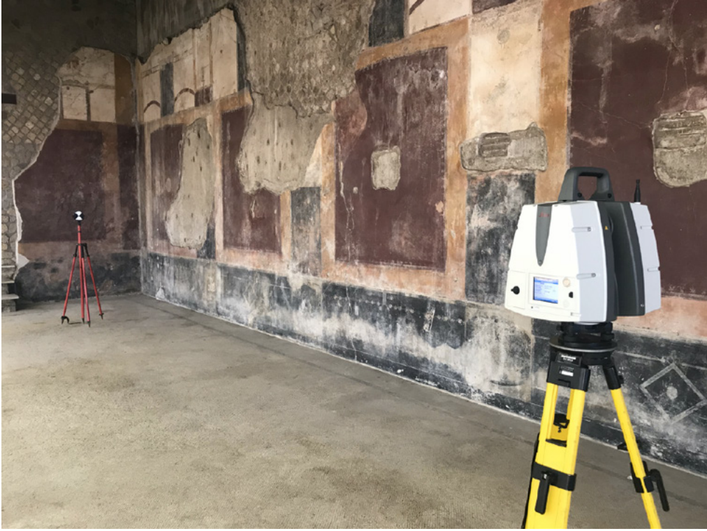
Figure 6. Csatellammare di Stabia. Villa San Marco. Leica P30 laser scanner being acquired (photo by the author).
