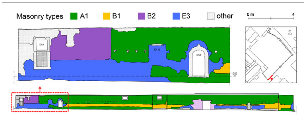
Figure 4. South-east frontage (PR2). detail and main masonry types. The most ancient structures are indicated through the codes 'B2' (Phase 1, first half of the 13th century) and A1 (Phase 2, second half of the 13th century).
