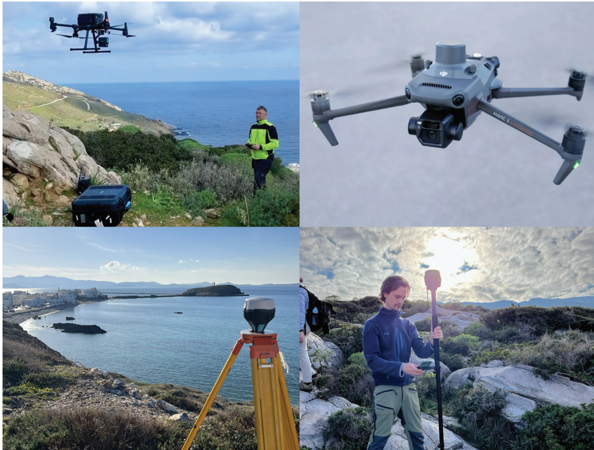
Figure 2. Equipment used for this study (clockwise from top left): DJI Matrice 300 RTK, DJI Mavic 3E RTK, Emlid Reach RS3 GNSS RTK as a rover for field survey, Emlid Reach RS2 GNSS RTK as a base
